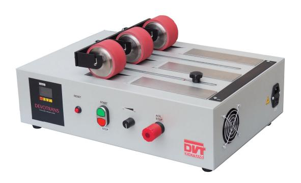
USED TO STICK BAND SAMPLES TO PREPARE THEM FOR TEST
